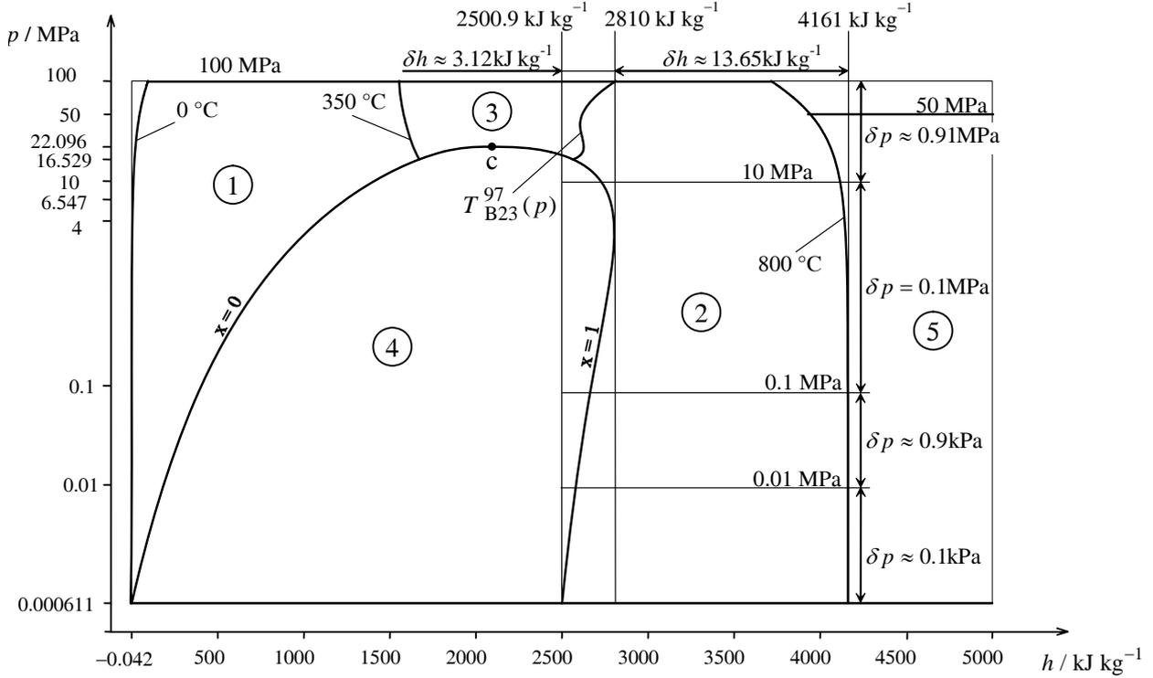
**Figure 3:**  $\lg p$ - $h$ -diagram with sub-divided  $p$ - $h$  grid according to Table 1, where  $\delta p$  and  $\delta h$  indicate the distance along  $p$  and  $h$ , respectively
